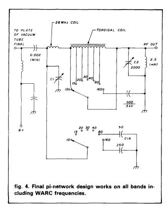
evaluating for the series capacitance how close we come to the required 340 pF.  $\frac{2400 \times 400}{2400 + 400} = 342.9$  pF.
